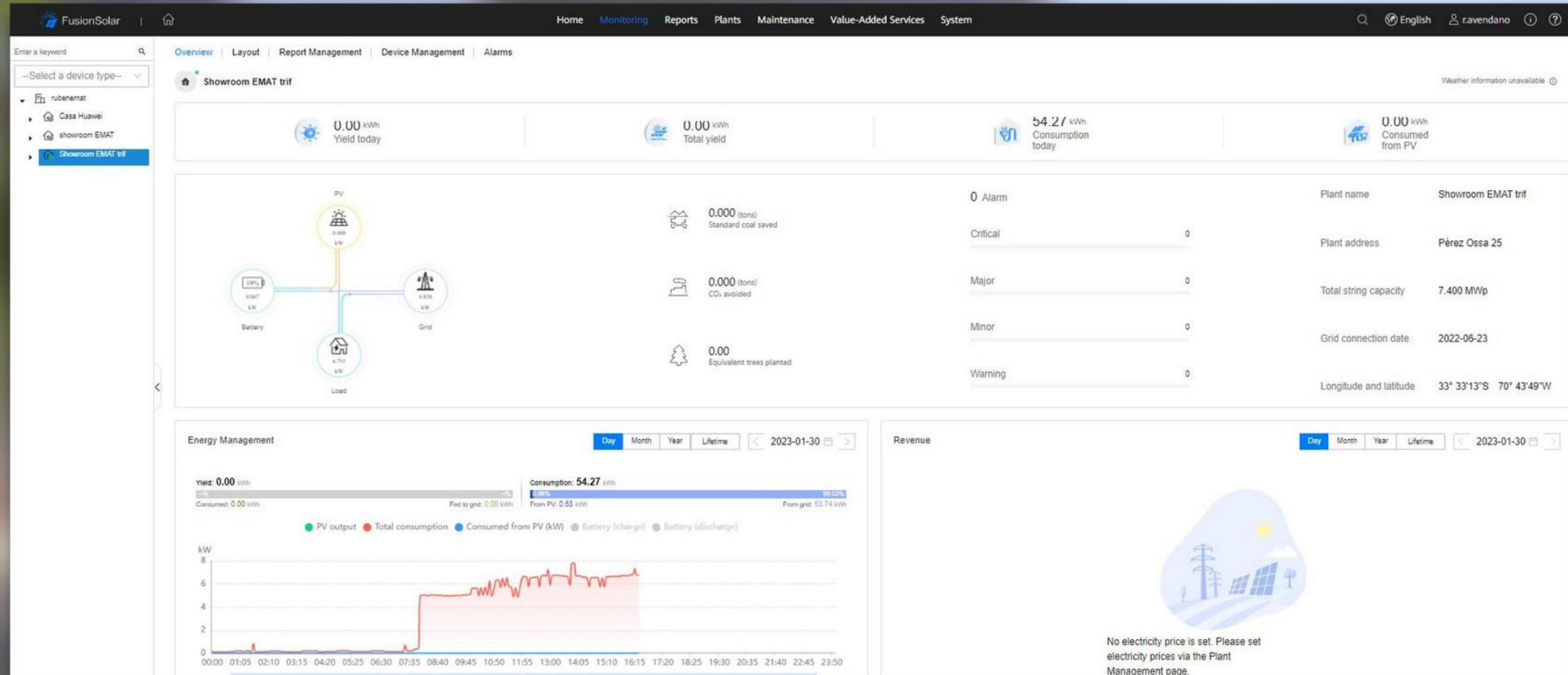
The screenshot shows the FusionSolar monitoring interface for a plant named 'Showroom EMAT trif'. The dashboard includes a navigation menu, a search bar, and several key performance indicators (KPIs) for the current day (2023-01-30):
