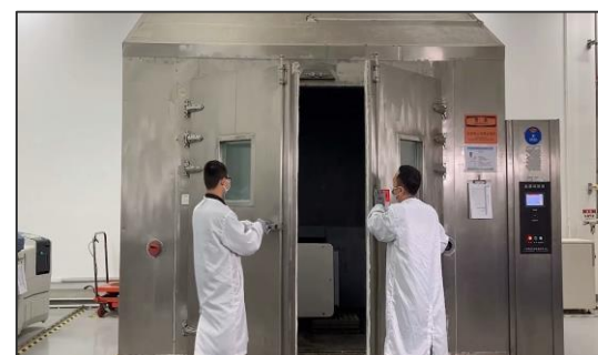
Salt spray test chamber
