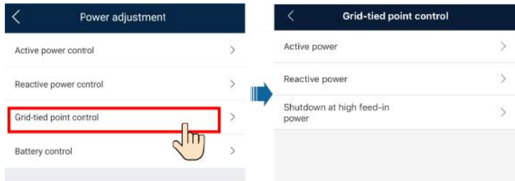
Figure 7-7 Grid-tied point control
