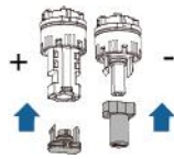
Figure 5-16 Sealing plugs with snap-fits
