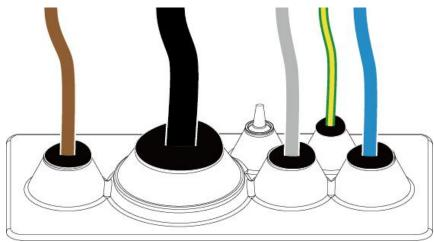
**Step 3** After cables are installed, seal the cable holes for power cables and communications cables using the delivered sealing putty.
