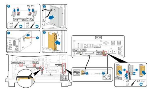
Figure 7-9 SmartLogger cable connection 1
