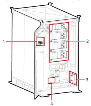
Figure 2-12 Positions of monitoring system components
