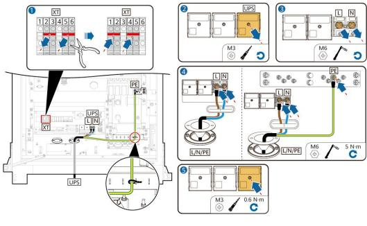
Figure 7-4 Connecting UPS cables
