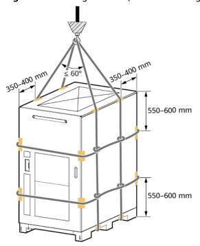
Figure 6-5 Moving the ESS (method 2: using endless slings)
