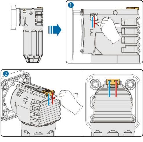
Figure 7-15 Marking alignment lines to confirm proper installation (model 2)
