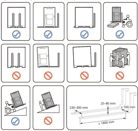
Figure 6-6 Moving the ESS (method 3: using a forklift)
