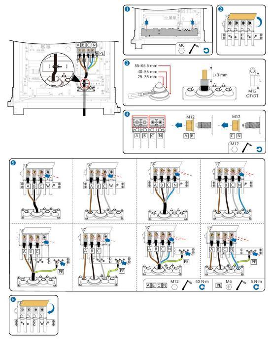
Figure 7-1 Installing PCS power cables
