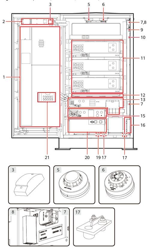
Figure 2-5 Components (interior view, with DCDC)
