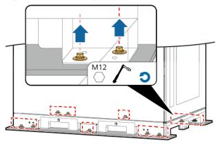
**Step 4** Remove the forklift positioning plates.
