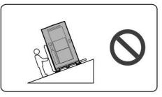
斜面禁止使用手动叉车搬运 Do not use a manual pallet truck to transport the cabinet on a slope.
