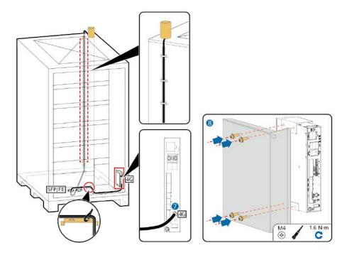
Figure 7-10 SmartLogger cable connection 2
