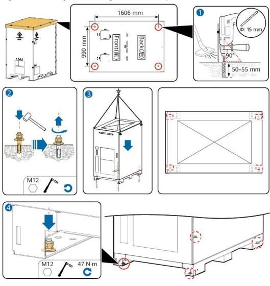
Figure 6-9 Securing the ESS using hidden screws (plan 3)
