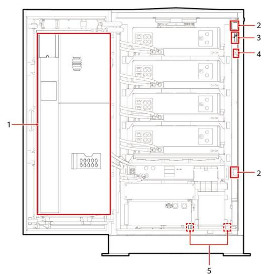
Figure 2-15 Position of the environment control system
