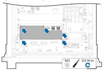
Figure 7-16 Installing the RCM cover
