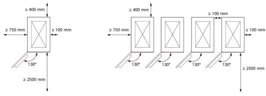
Figure 5-2 Clearance requirements (2)
