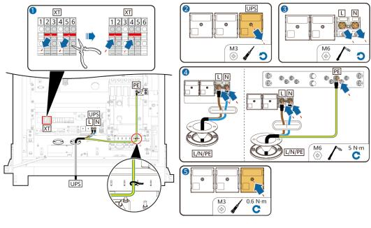
Figure 7-4 Connecting UPS cables
