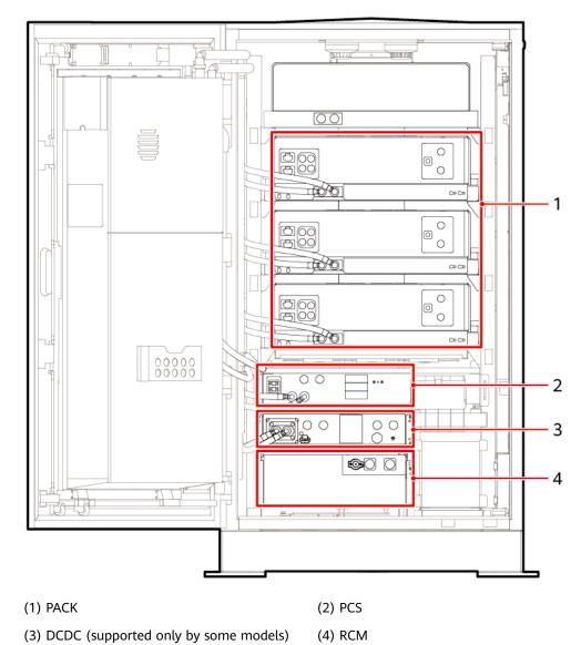
Figure 2-6 Position of the power supply and distribution system
