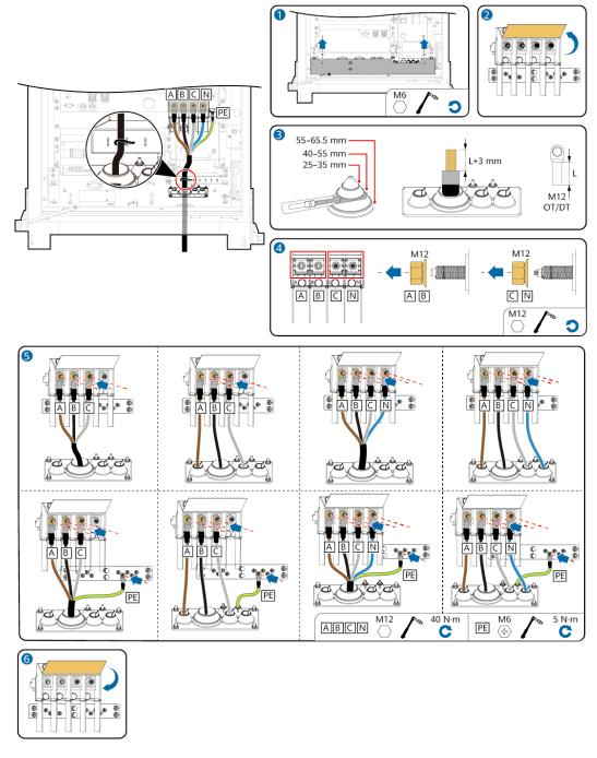
Figure 7-1 Installing PCS power cables
