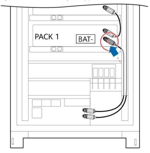
Figure 7-11 Position for connecting a battery pack cable
