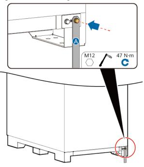
Figure 6-10 Grounding outside the cabinet (flat ground bar)
