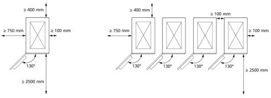
Figure 5-2 Clearance requirements (2)
