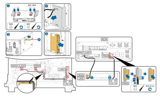
Figure 7-9 SmartLogger cable connection 1
