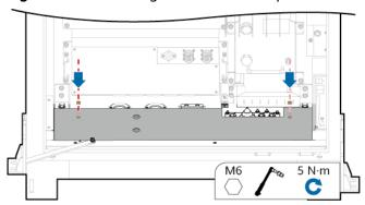
**Step 5** Reinstall the external bottom baffle plate for the ESS.
