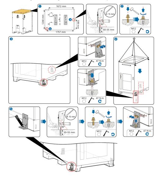
Figure 6-8 Securing the ESS using three anchor brackets (plan 2)
