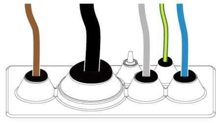
**Step 3** After cables are installed, seal the cable holes for power cables and communications cables using the delivered sealing putty.
