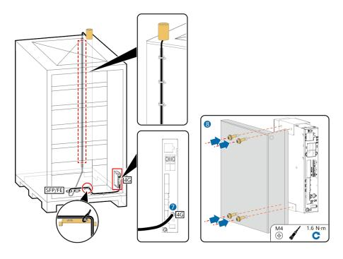
Figure 7-10 SmartLogger cable connection 2
