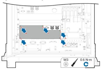
Figure 7-16 Installing the RCM cover
