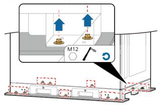
**Step 4** Remove the forklift positioning plates.
