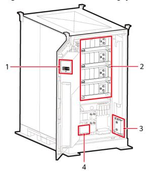
Figure 2-12 Positions of monitoring system components
